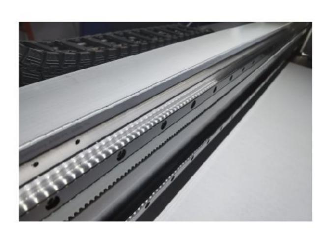
High stability imported magnetic encoder strip is more durable, improving the printing stability and ensuring a high-quality continuous output
