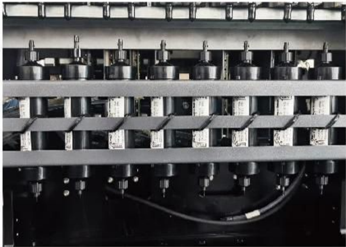
Air degassing unitIt removes micro bubbles in inkwhile transferring ink to main ink tank
