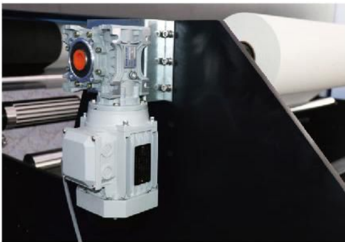
Frequency motor ensures more stable material loading and take-up
