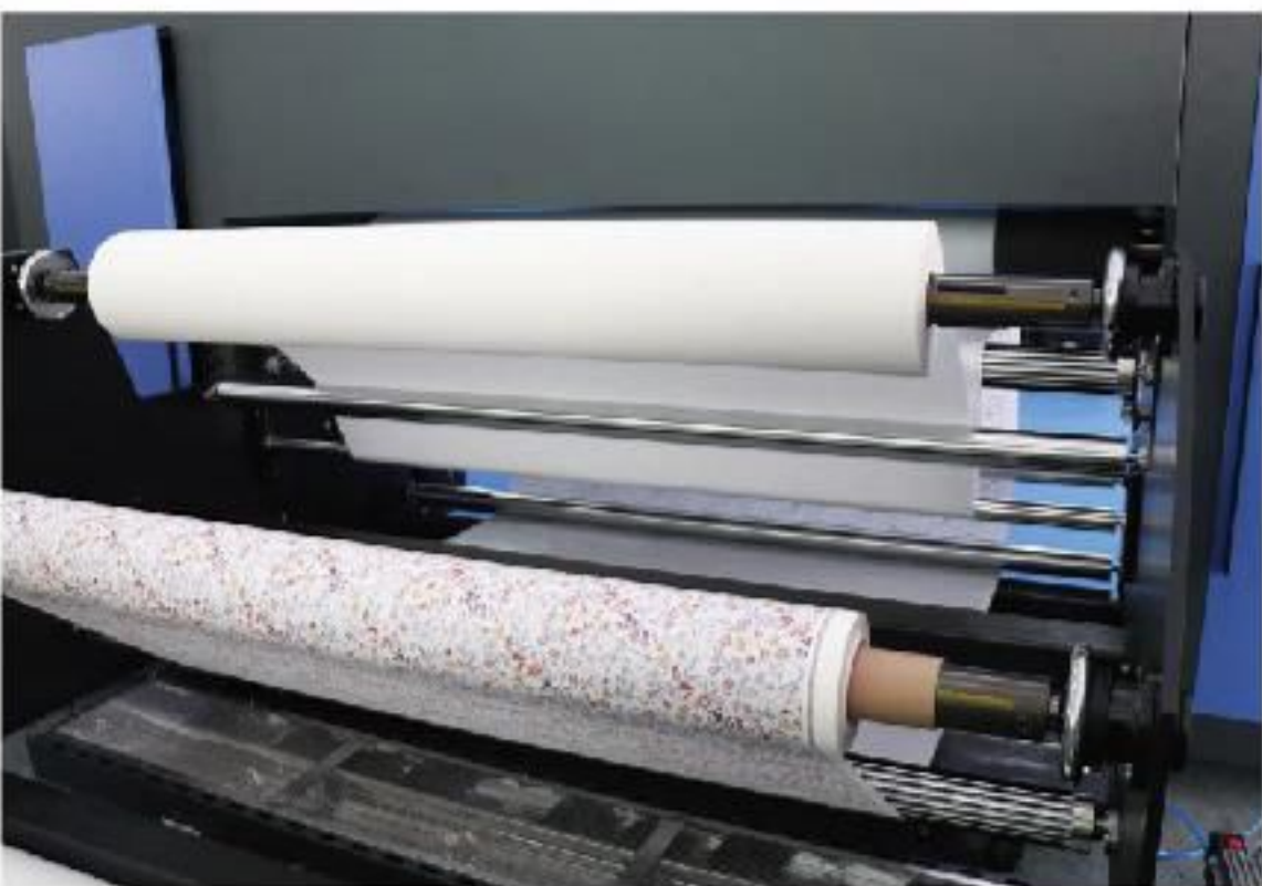
Rear loading and take-up to facilitate workflow
