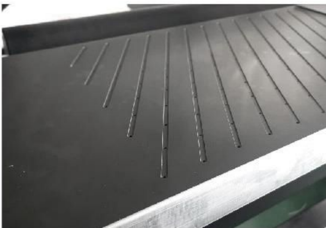
Honeycomb suction platform, less deformation during paper moving, print width up to 2050mm
