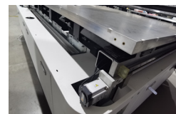
The new Y-direction adopts Panasonic dual servo motor, and the old single motor with double belt structure, comparison: the new transmission is more accurate
