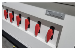
The new model has six suction zones for a wider selection of zones
