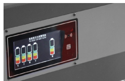
Ink level display + alarm system, humanized design, monitor ink usage at any time
