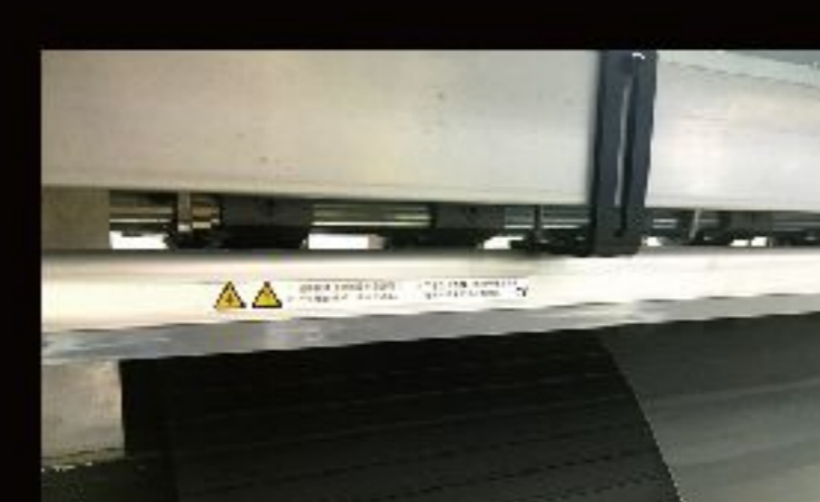
Anti-static device equipped to fight against static and ensure accurate ink droplets positioning
