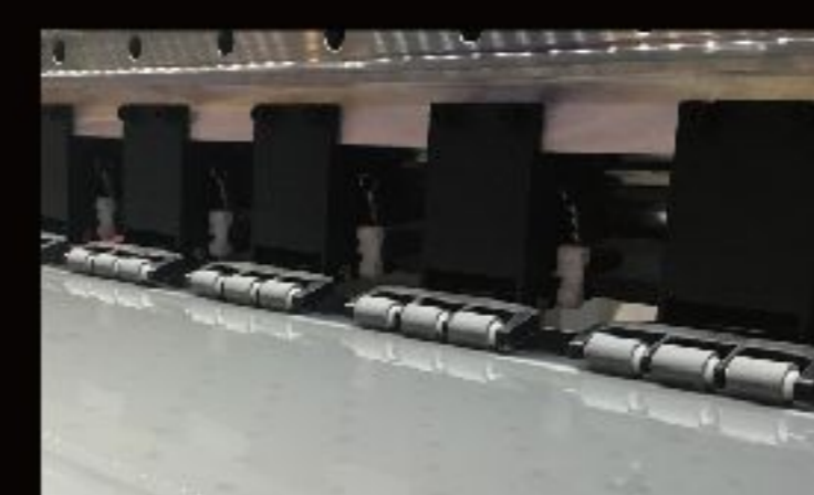
More stable feeding system with 3-foot pinch rollers
