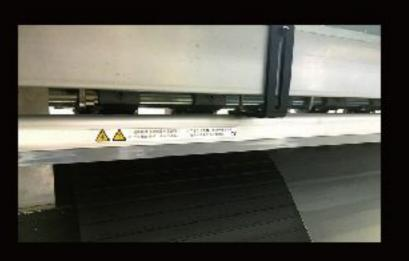
Anti-static device equipped to fight against static and ensure accurate ink droplets positioning
