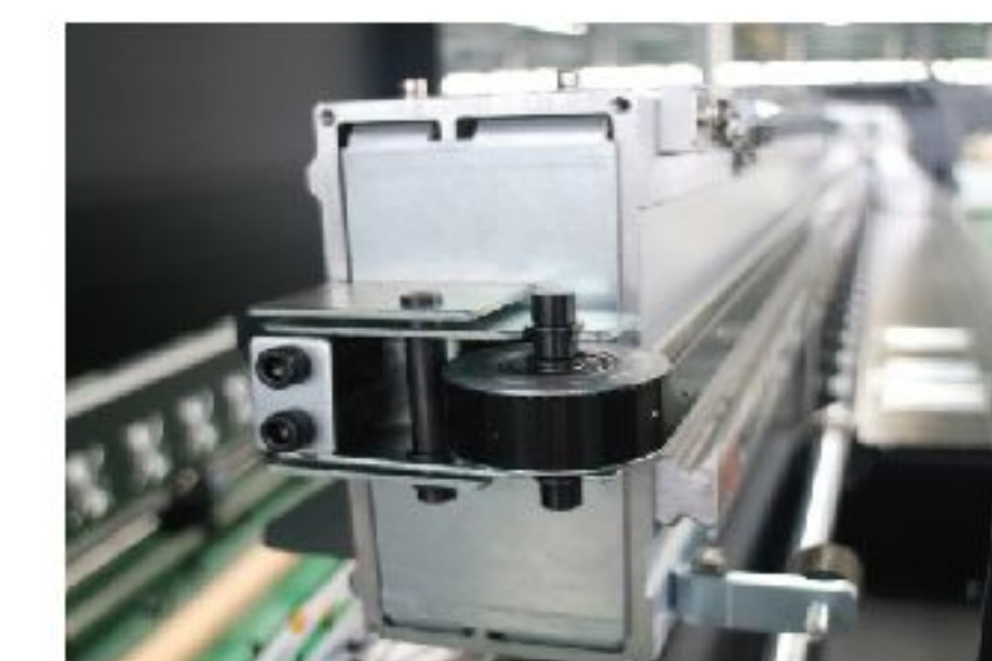
High-precision and high-stability tensioning pulley system.
