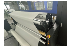
The special feeding system for fabrics can adapt to cotton fabrics of different thicknesses
