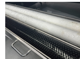
Equipped with a belt-guided sponge brush, it can be cleaned while printing to ensure that the fabric is clean and tidy during the printing process
