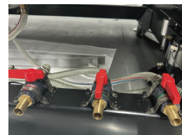
The guide belt is equipped with water-based function to ensure that the fabric is clean and also can adapt to more ink application solutions
