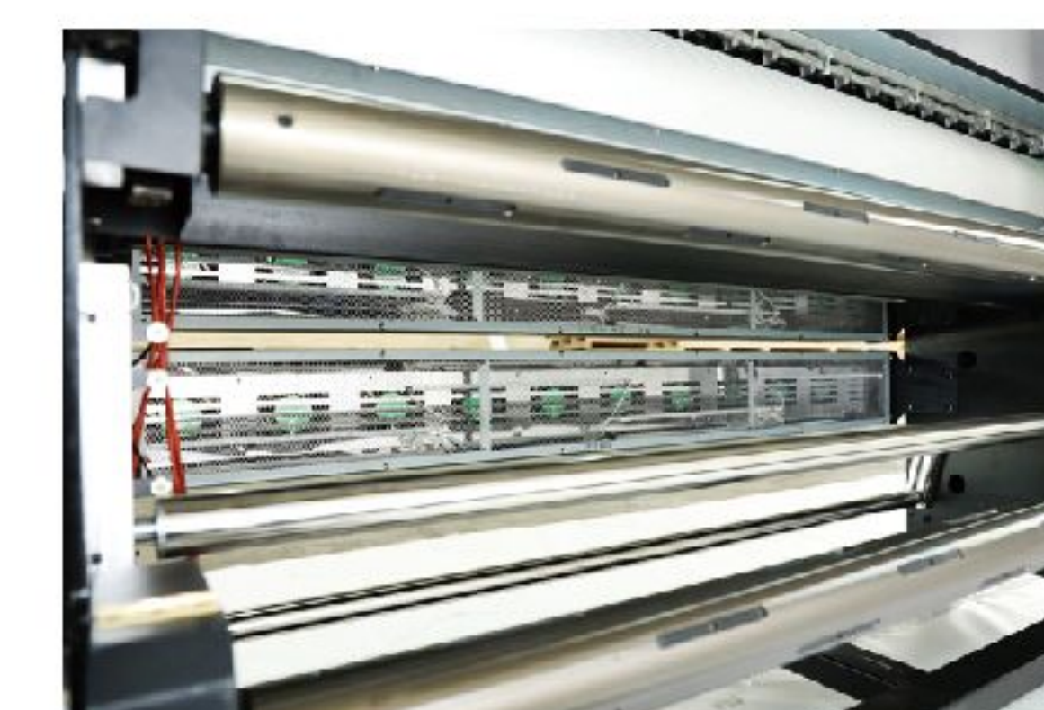
Inflatable take up and feed media shaft.
