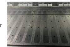
Vertical air guiding platform makes the paper surface flat
