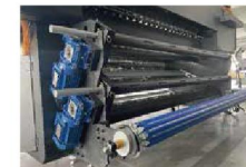
The air shaft take-up with rubber strip ensures stable media movement
