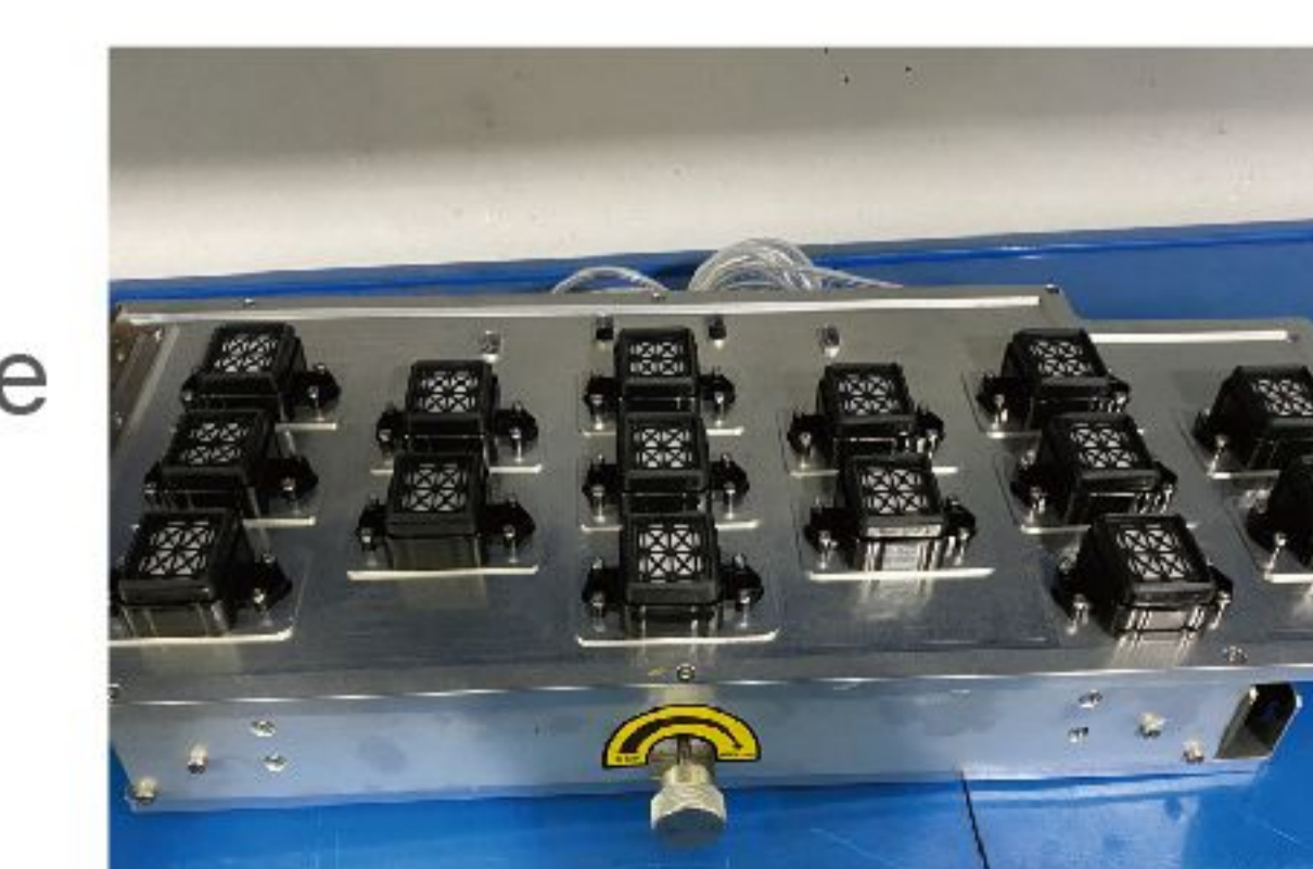
Captop and integrated wiper to moisturize heads, make it convenient for operation and maintenance
