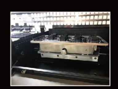
Automatic moisturizing capping station eases operation and maintenance
