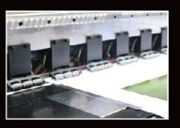
Height-adjustable pinch rollers with multiple feet
