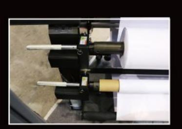
Air shaft take-up and loading system supports heavy media
